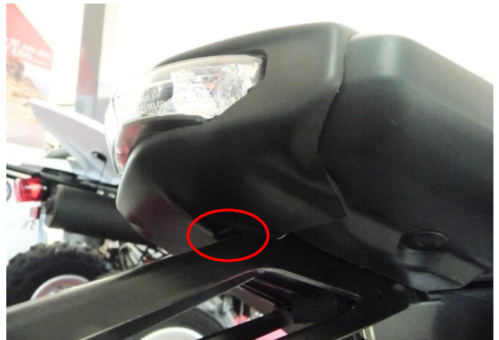
Fitting location of the tail light surround
