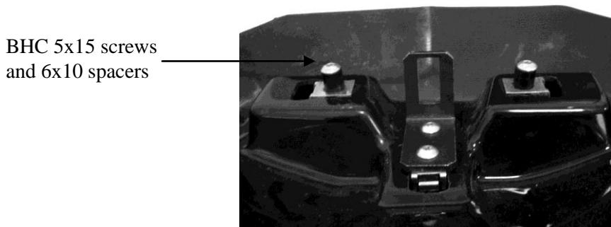
Before tightening completely, place the seat cover on the bike, center it (move the position of fasteners if necessary), remove it and tighten screws so as to block the fasteners location.
